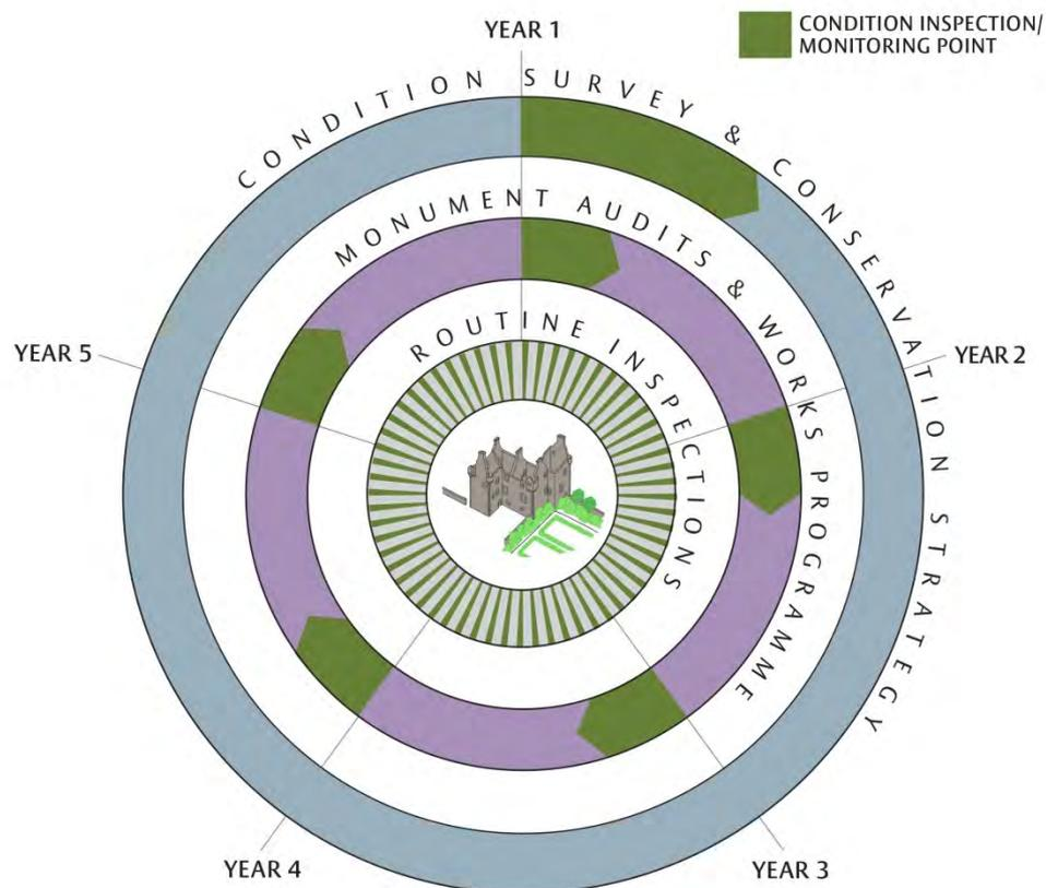
The green arrows indicate all the Condition Inspection and monitoring points over a typical 5 year period:
