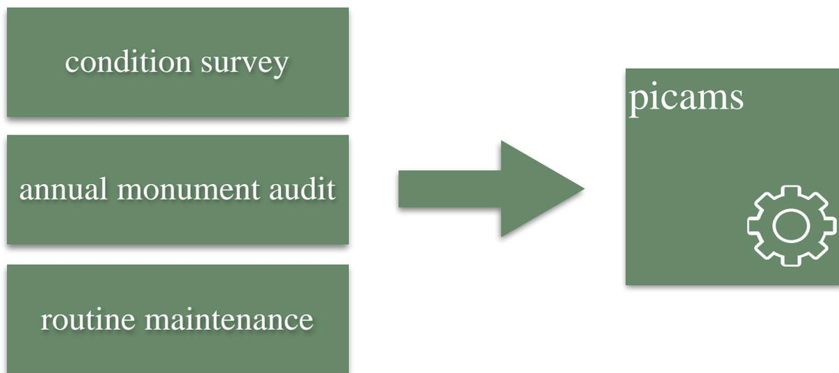
The system comprises a field data capture tool that transfers all current condition data into a single dynamic database, that can be accessed and interrogated by whatever reporting format is required for a particular purpose at a particular point in time.
